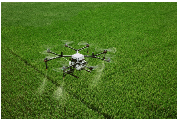
Fig. 1 A crop-dusting drone spraying a field for precision agriculture. Image by DJI-Agras from pixabay.com
