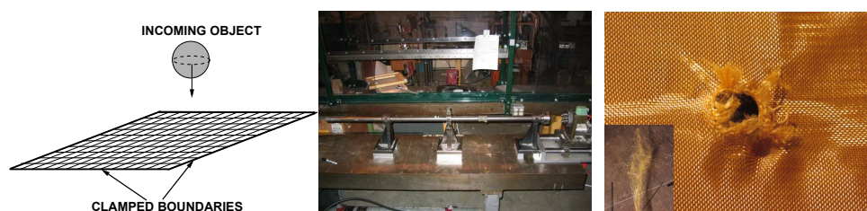
Fig. 1 (online colour at: www.gamm-mitteilungen.org ) LEFT: A schematic of the impact scenario. MIDDLE: UC Berkeley facilities Pneumatic gun-breech and barrel set up (top right, photo courtesy of D. Powell). Post impact puncture of Zylon target. Insert : The yarn comprising Zylon.
